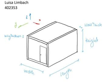
Volume = (Width-2\*WallThickness)\*(Length-2\*WallThickness)\*(Height-2\*CeilingThickness)
